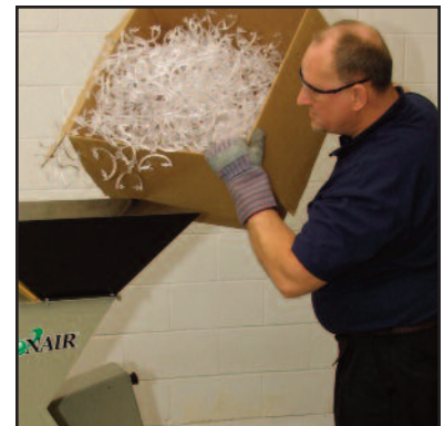
Don't overfeed your granulator. Consistent feeding of scrap decreases downtime.
