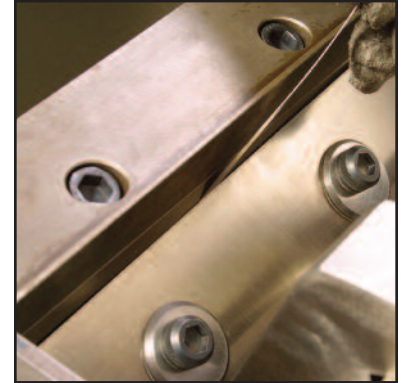
To ensure quality regrind, maintain the proper gap between the rotating knives and bed knives.
